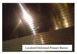
Figure 1-4: Permanent deformation in the primary barrier due to sloshing [21]
