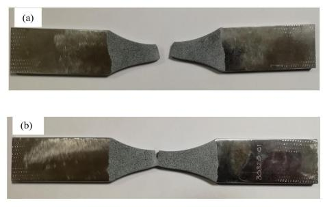
Figure 4-22: (a) Third specimen at the end of test (b) Fourth specimen at the end of test.
