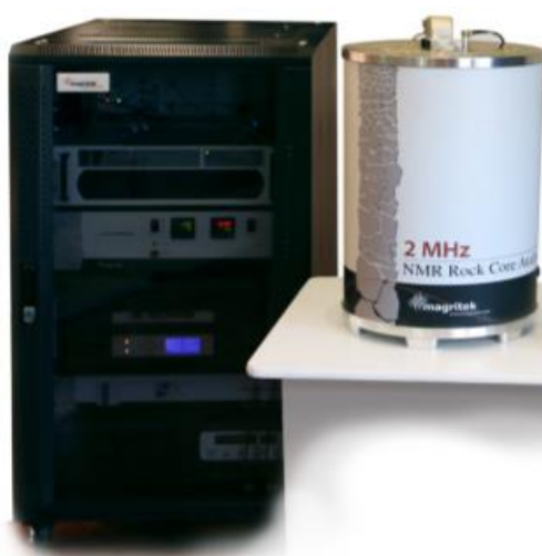
Figure A2-1: Magritek 2MHz NMR Rock Core Analyzer
