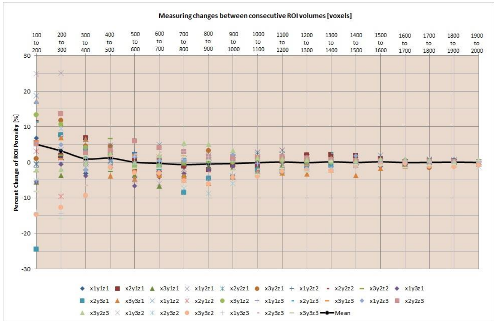
Figure 5-12: Identifying the REV at the Automatic Threshold Value for the Berea Sample using a Percent Change Approach
