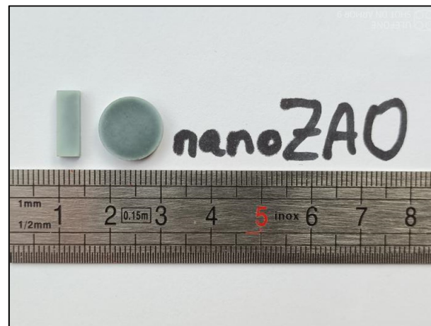
Figure 1. A set of typical \text{Zn}_{0.995}\text{Al}_{0.005}\text{O} samples (nanoZAO composition) prepared via aluminothermic reactions and used in the different analyses performed in this work.
