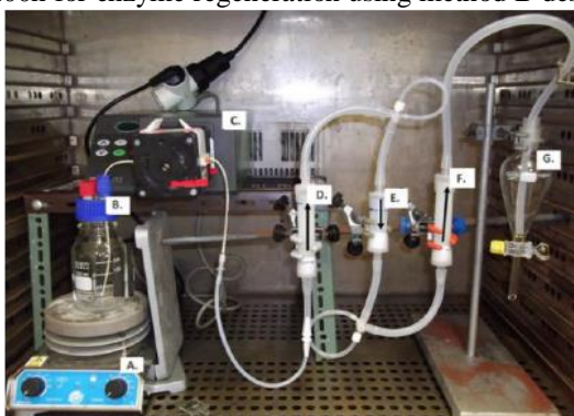
Fig. 1 Experimental apparatus for the continuous-regime experiment. A – stirring device; B – Feed mixture; C – Pump for reactional mixture feeding; D – 1 st fixed bed bioreactor; E – Resin column; F – 2 nd fixed bed bioreactor; G – Sampling point.
