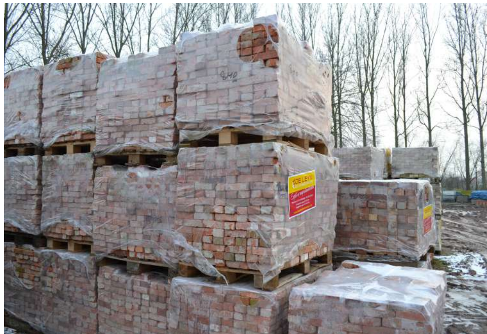
Overview of the stock of a dealer in reclaimed bricks. This company has a permanent stock of almost one million bricks (De Leyn Bouwmaterialen, Moerkerke, Belgium).
