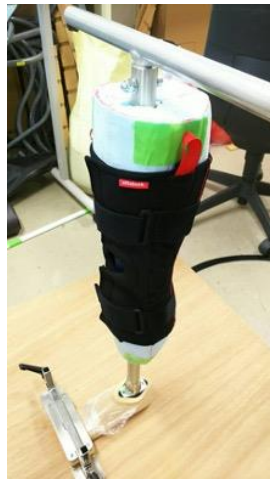
Figure 4. 17 Artificial Leg for Simulating Knee Flexion
