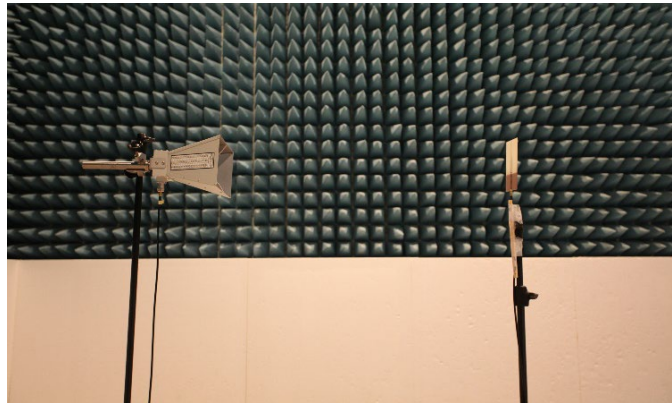
Fig. 6.12 Experiment setup for transfer function and antenna factor
