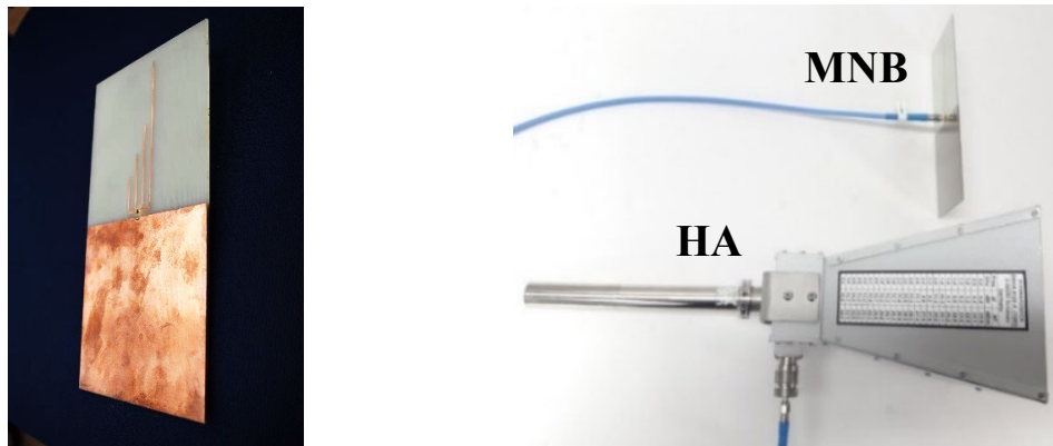
Fig. 3.21 Comparison of size and shape between the fabricated four strips MNB antenna and a Horn antenna (HA)
