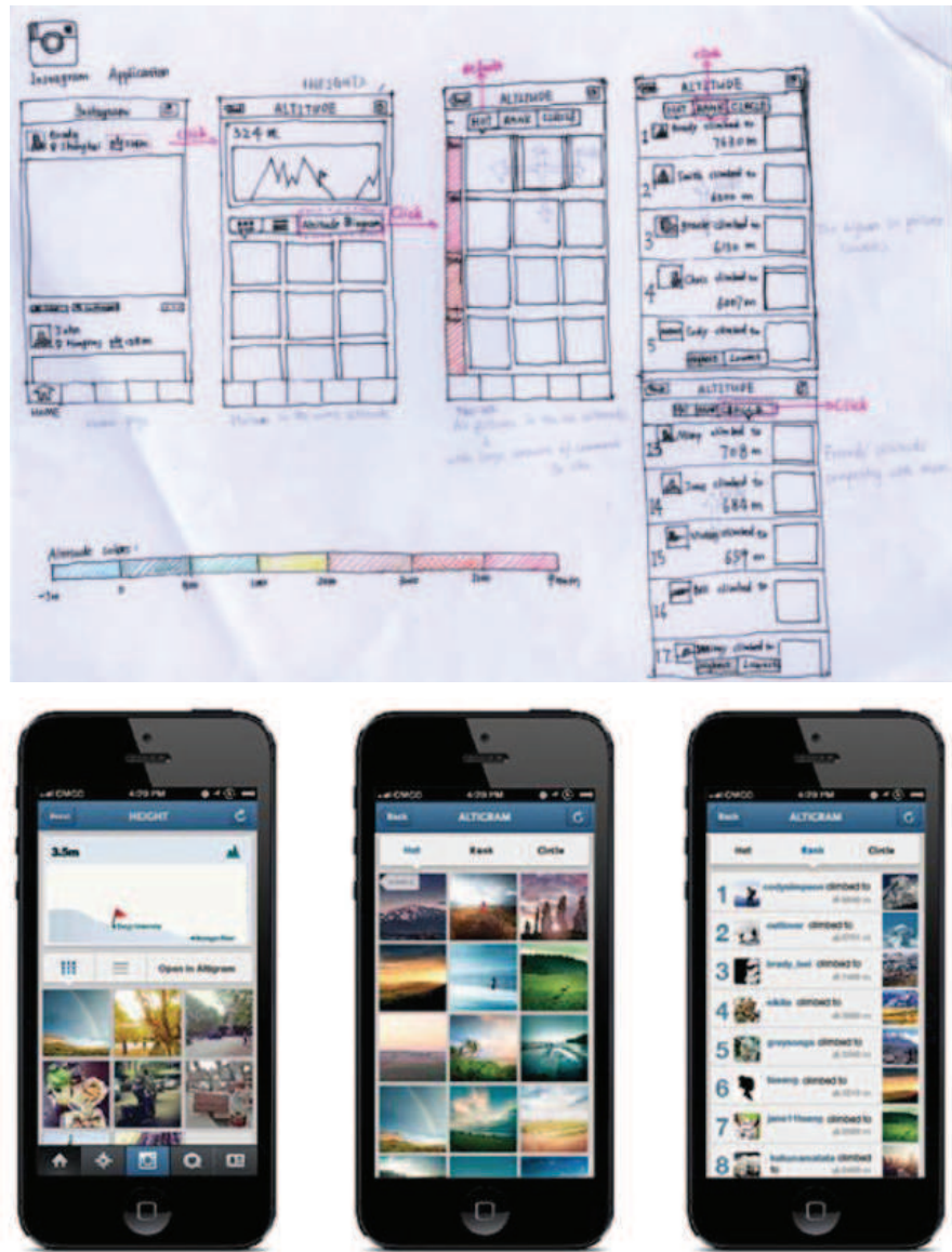
Figure 9 On the left we see the visualization sketches for Altigram app in the smart phone device. And on the right we see the detailed design of the same visualizations. Note how the color strip envisioned initially was removed in the final design (used with permission of students)
