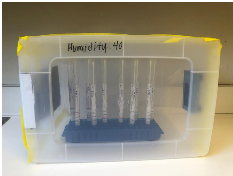
Figure 5.7. Type two box of relative humidity 35% on the modern lab counter
