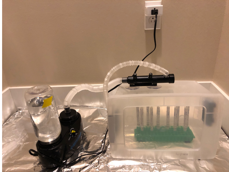
Figure 5.8. Type two box of relative humidity 50/60% in enclosed closet with aluminum foil underneath.
