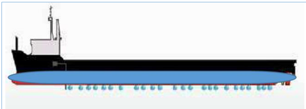
Figure 31 Micro-Bubble Air Lubrication (Source: (SN & S., 2018))
