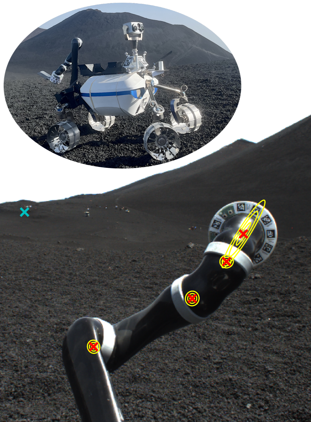
Figure 1: Our LRU rover on Mt. Etna. PK-ROKED detects keypoints on the Jaco2 arm: Detected keypoints , corresponding uncertainty ellipses , and detected false positives .
