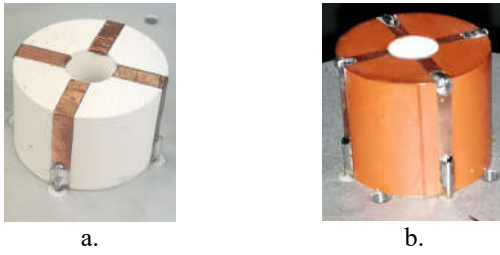
Figure 1. 3D printed ceramic cylindrical dielectric resonator antennas (DRA). (a.) DRA with copper feed-strips. (b.) DRA with feed-strips on an adhesive Kapton polyimide sheet.
