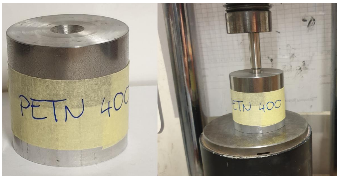
Figure 1. Experimental setup consisting of an aluminum block and steel block with hole connected by crepe tape (left), test setup during the pressing process (right).
