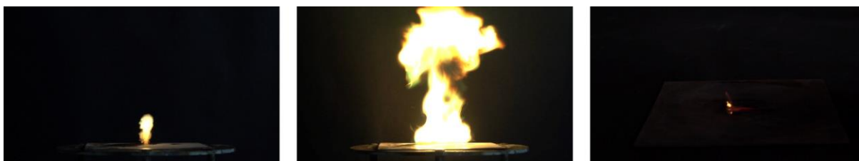
Figure S10. Reactions of [\text{Cu}(\text{AMT})_4(\text{NCA})](\text{NCA}) ( 9 ) during hot plate test (left & middle) and hot needle test (right).
