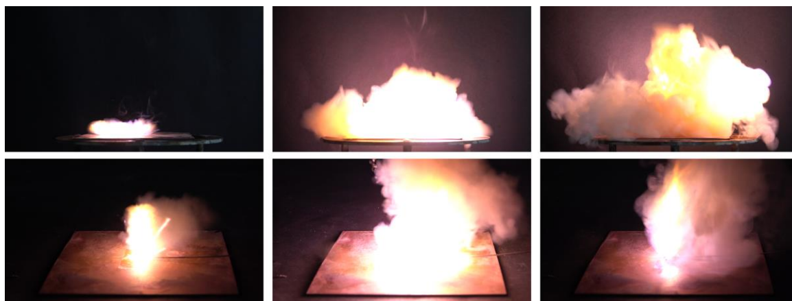
Figure 16. Deflagration of silver nitrocyuanamide ( 5a ) during hot plate (top) and hot needle tests (bottom).
