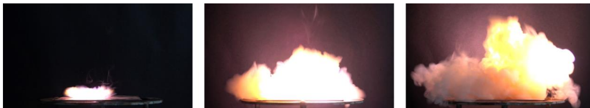
Figure S8. High-speed images of the deflagration of silver nitrocyanimide ( 6a ) during the hot plate test.
