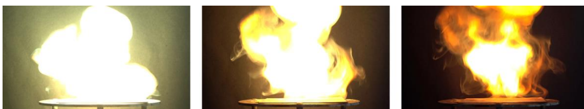
Figure S11. Deflagration of [\text{Cu}(1,1\text{-dtm})_2(\text{NCA})_2] ( 10 ) during hot plate test shown as a sequence.
