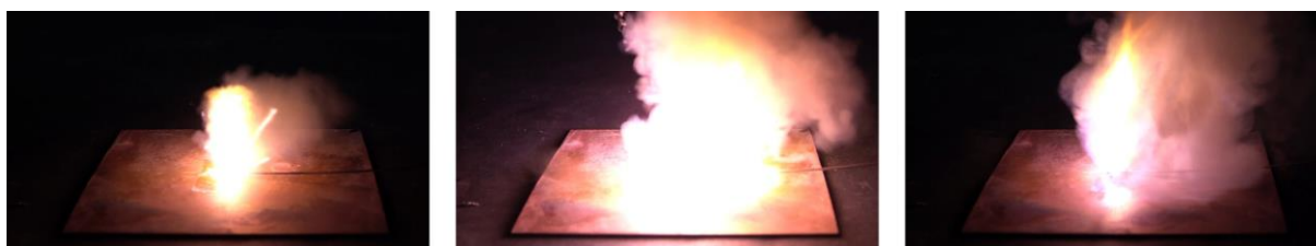
Figure S9. Deflagration of silver nitrocyanimide ( 6a ) during the hot needle test shown as a sequence.
