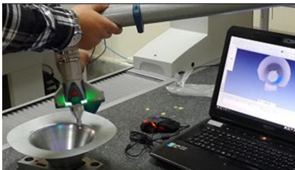
Figure 4. Laser 3D scanner with its associated software.
