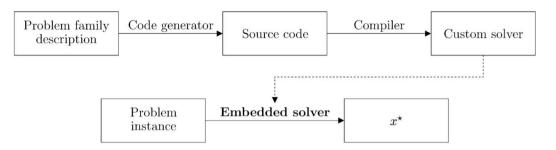
Figure B.1: The process of generating a custom solver in CVX/CVXGEN.
