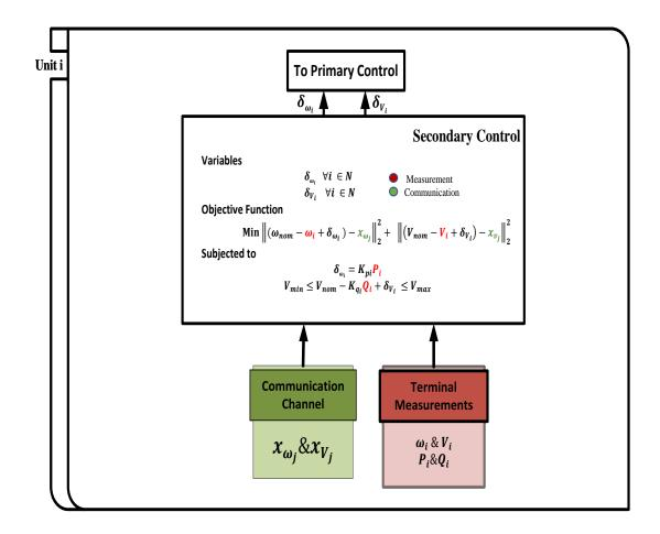
Figure 4.6: Optimization-based consensus secondary control.
