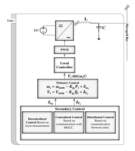
Figure 4.1: Grid-forming unit in the hierarchical control structure.
