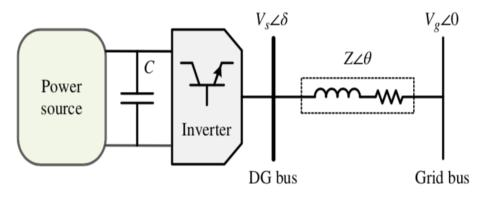
Figure 3.2: Inverter-based unit connected to a grid bus.
