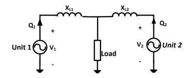
Figure 4.3: Two units are supplying a common load.
