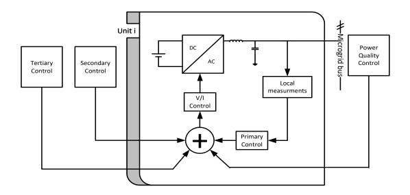
Figure 2.6: Hierarchical control structure.
