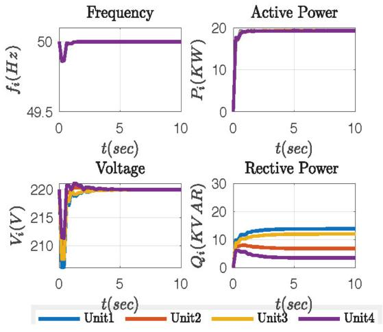
Figure 5.5: Decentralized secondary controller.
