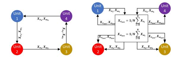
(a) Consensus-based communication topol- (b) Centralized-based communication topology. ogy.
