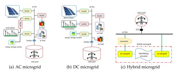
Figure 2.2: Microgrid architectures.
