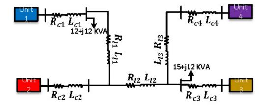
Figure 5.3: Single-line diagram of the microgrid test system.
