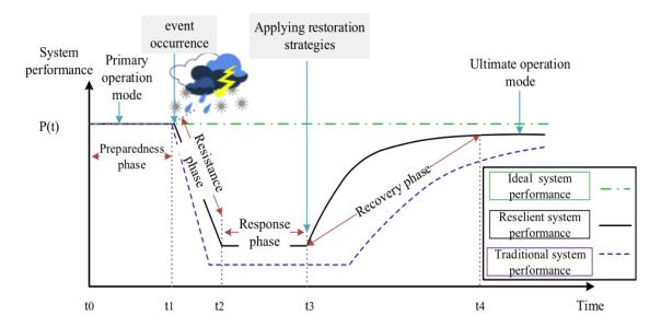
Figure 2.1: The performance levels of a resilient power system in the face of a disruptive event.
