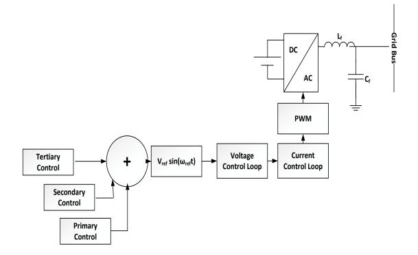
Figure 3.1: The hierarchical control structure of grid-forming units.
