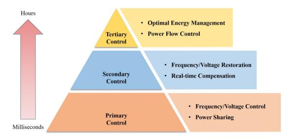
Figure 1.4: The hierarchical control structure.
