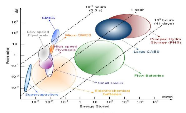
Figure 2.3: Power and energy densities of different energy storage devices.
