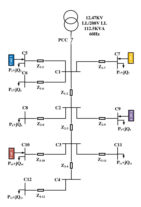
Figure 6.1: The modified commercial feeder of LV North America distribution system benchmark.
