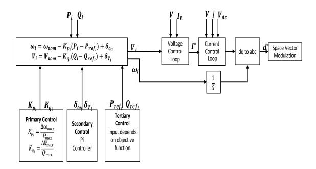
Figure 5.1: Hierarchical control structure.
