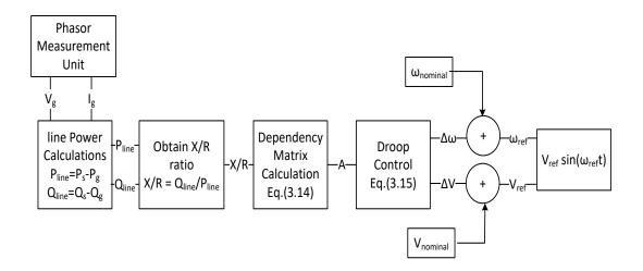
Figure 3.3: The block diagram of the proposed droop controller.
