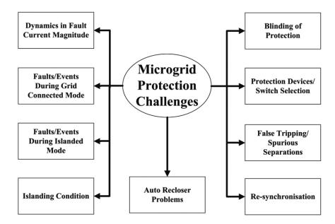
Figure 2.5: Challenges in protection associated with AC microgrids
