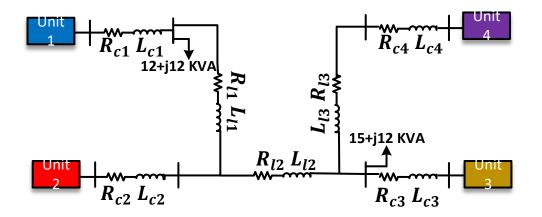
Figure 4.7: Single-line diagram of the microgrid test system .
