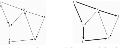
(a) A directed graph.(b) Spanning tree in the directed graph.Figure A.1: An example of a directed graph.
