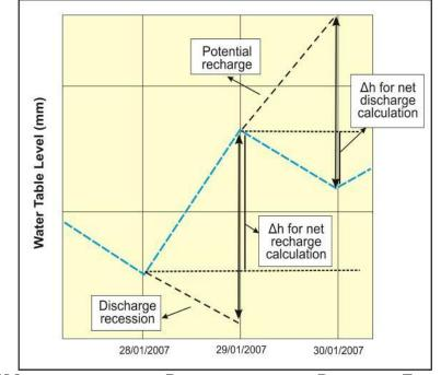
FIG. 7 MEASUREMENTS TO BE PERFORMED FOR THE DISCHARGE ESTIMATION
