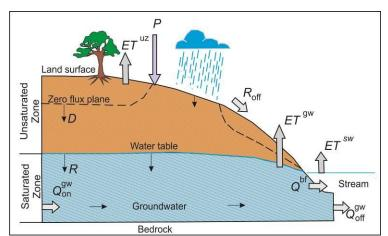
FIG. 5 DIAGRAM THROUGH A WATERSHED SHOWING WATER BUDGET COMPONENTS AND DIRECTIONS OF WATER MOVEMENT [2]
