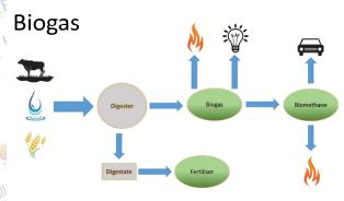
Biogas is produced from organic material break down, with different percentage levels relative to the feedstock used.
