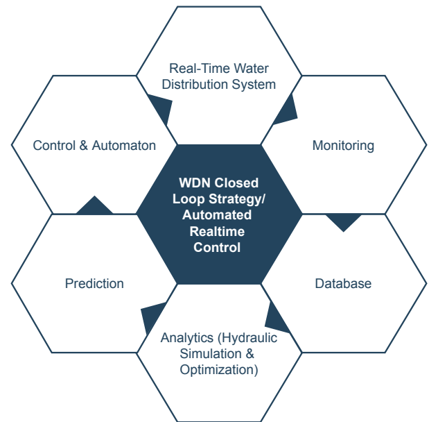
FIGURE 3. Closed-loop strategy for water supply system.
