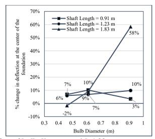
Figure 2.6. Effect of bulb diameter, with 1.22 m roots at various shaft lengths
