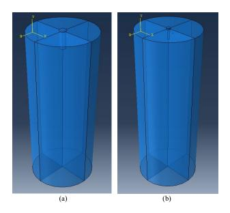
Figure 2.1. (a) Conventional foundation embedded in soil (b) RFS system embedded in the soil
