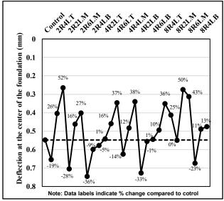
Figure 3.5. Overall summary of deflection data obtained from the 27 models developed in this research along with the control
