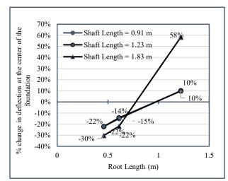
Figure 2.5. Effect of root length for a 0.91 m bulb diameter
