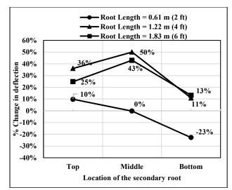
Figure 3.8. Variation of % change in deflection with the location of the secondary root and its length for the root-foundations with eight roots
