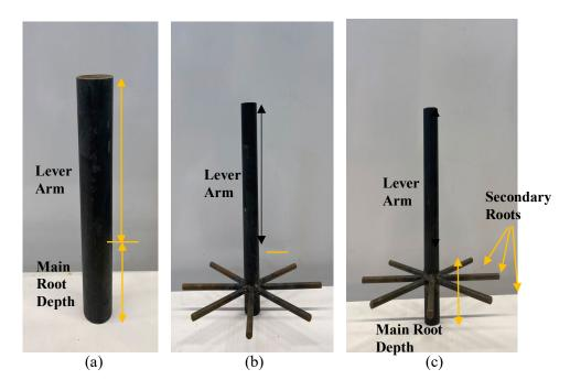
Figure 4.5 Physically Tested Foundation Systems (a) Control (b) S-6LM (c) S-6LT
