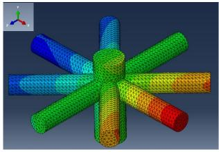
Figure 3.4. Deformed mesh of the 8-root foundation model
