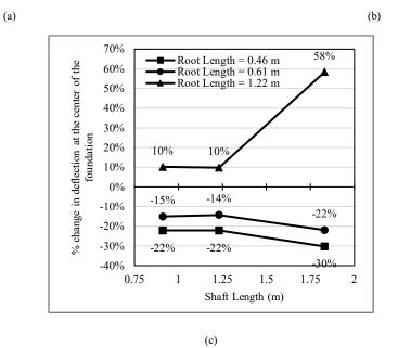
Figure 2.4. Effect of shaft length (a) 0.46 m bulb diameter, (b) 0.61 m bulb diameter, (c) 0.91 m bulb diameter
