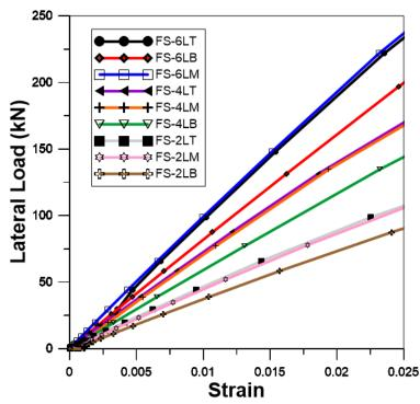
Figure 4.3 Lateral Load vs Strain Plots for the Nine Preliminary RFS Models Comparison
