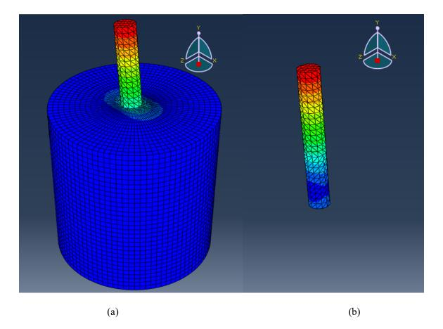
Figure 4.8 (a) Scaled Control Foundation Embedded in Soil (b) Scaled Control Foundation
