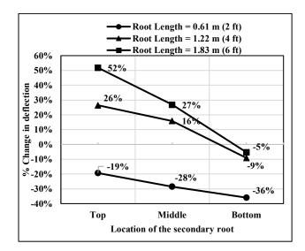
Figure 3.6. Variation of % change in deflection with the location of the secondary root and its length for the root-foundations with two roots
