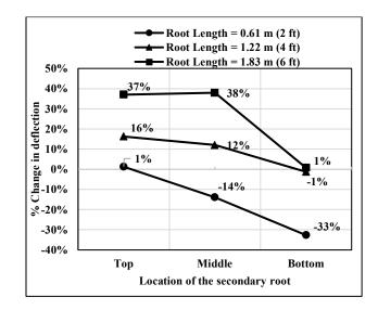
Figure 3.7. Variation of % change in deflection with the location of the secondary root and its length for the root-foundations with four roots
