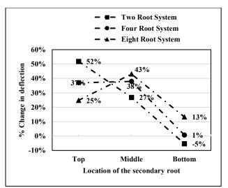
Figure 3.9. Variation of % change in deflection with the number and location of the secondary roots for the root-foundations with root length of 1.22 m
