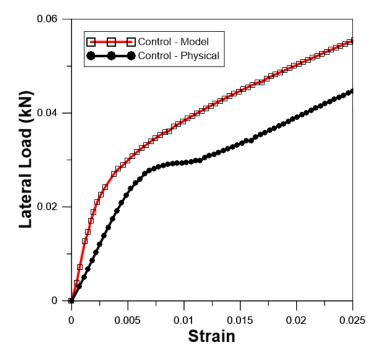
Figure 4.9 Control Physical and Model Lateral Load Capacity Comparison
