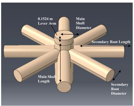
Figure 4.11 Schematic of a Typical Taproot-Inspired RFS
