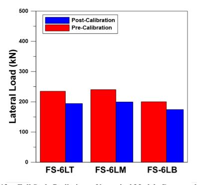
Figure 4.13 Full Scale Preliminary Numerical Models Compared to Full Scale Calibrated Numerical Models
