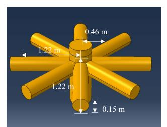
Figure 3.3. Typical root foundation with eight secondary roots at the top of the tap root
