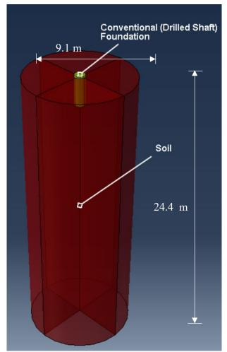
Figure 3.2. FEM model of the conventional foundation system
