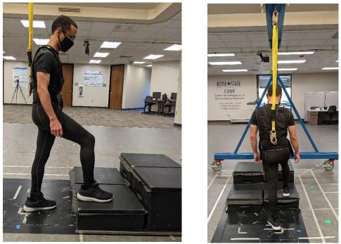
Figure 3.1 Weight supporting gantry used for stair ascent and stair descent task
