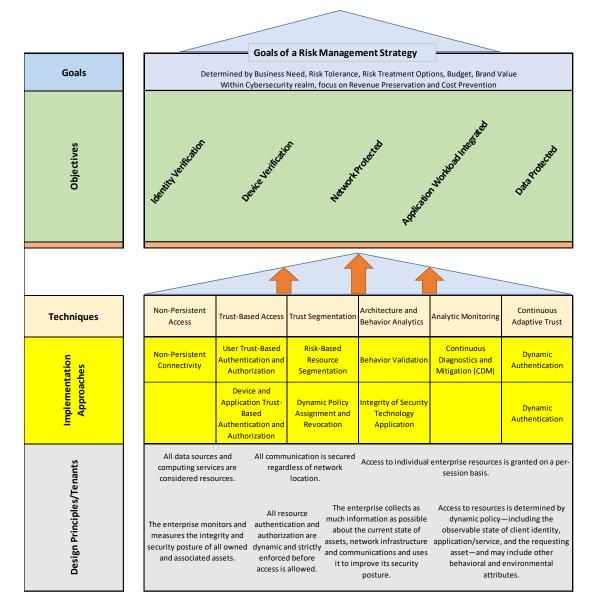
Figure 1: Applying CISA Cyber Security Model with NIST Cyber Resiliency Constructs to Implement Zero Trust Architecture
