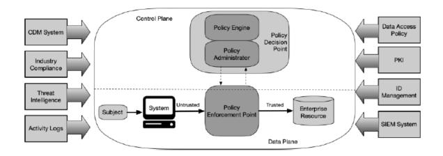
Figure 2: Core Zero Trust Logical Components [NIST SP 800-207]
