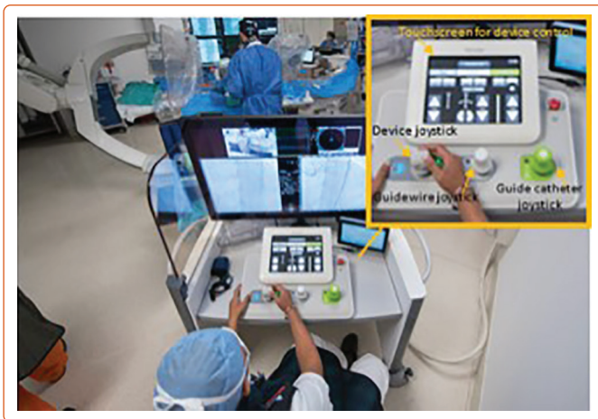
The general setup of our robotic percutaneous coronary intervention cases at the Cleveland Clinic. One of the interventional cardiology operators sits in the cockpit to control the robotic arm, while the other is at bedside to assist with device exchanges and manipulation of the image intensifier.
