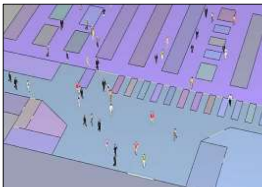
Figure 6 - Simulation moment for the first scenario, the first case, for occupant's speed of 0.95 m/s
