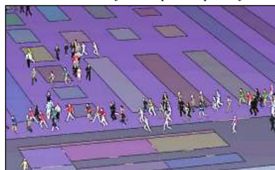
Figure 9 - Simulation moment for the third scenario, the second case, for occupant's speed of 1.2 m/s
