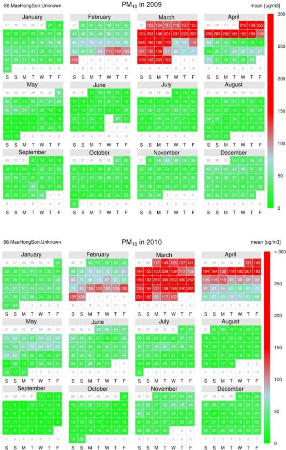
Figure 1 Calendars of PM10 concentrations (24-hour average values) from 2009 to 2014 of the Mae Hong Son station (ID.66).
