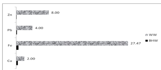
Figure 2 Coefficients KK of heavy metals in groundwater (boreholes and wells near textile mills in Ikorodu, Nigeria).
