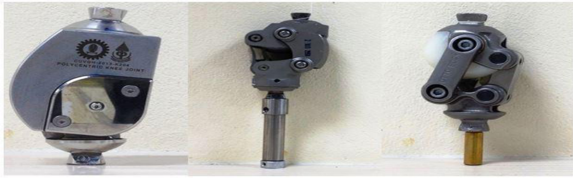
Fig 1. Image of three prosthetic knees tested: From left to right; Chulalongkorn University (CU) Polycentric Knee Joint, Prosthesis Foundation Knee, Otto Bock 3R20
