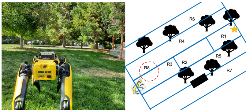
Fig. 2.5: Example of obstacle regions used for the machine learning to know where obstacles are. Onboard lidar can sufficiently cover a 360 degrees field of view.
