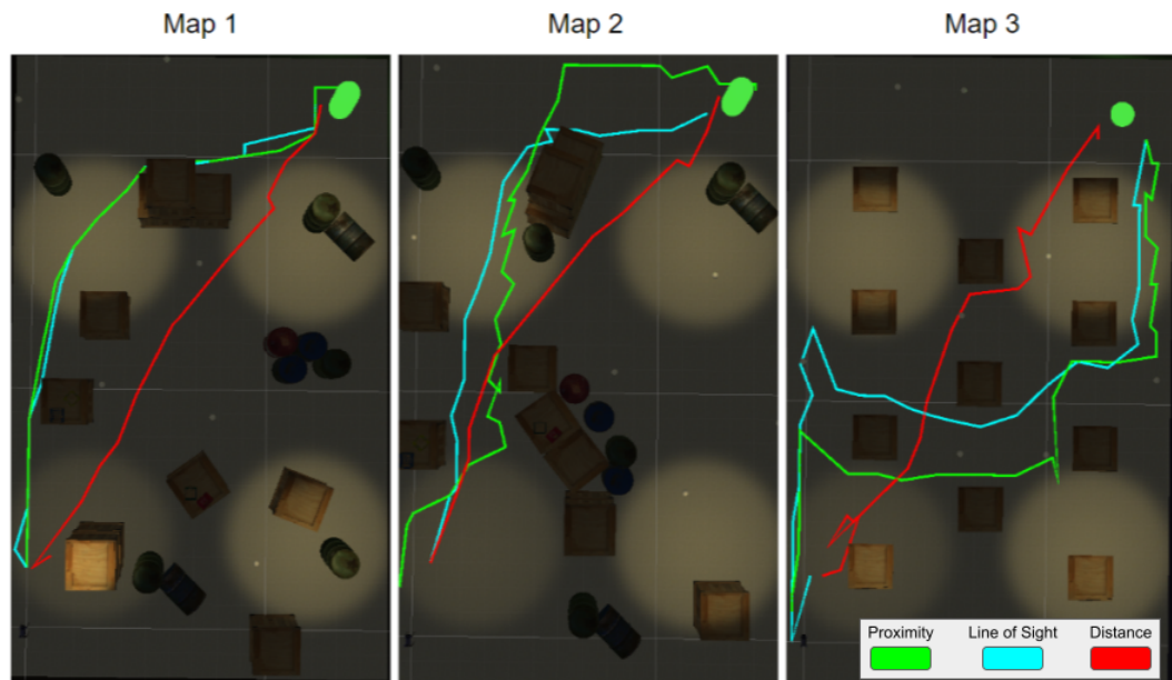
Fig. 3.6: Examples of the different heuristic paths. The distance path (in red) tends to move through open areas while the proximity (green) and line of sight (blue) avoid regions without occlusion.
