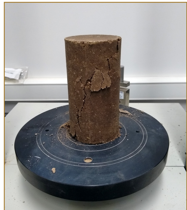
Cement treated specimen post Unconfined Compression Test
