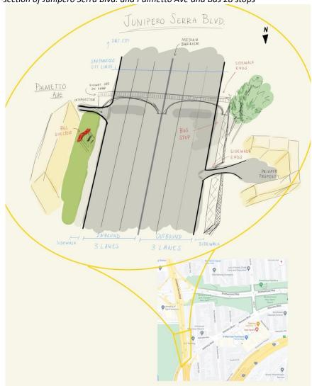
Figure 2-3: Cross-section of Junipero Serra Blvd. and Palmetto Ave and Bus 28 stops
