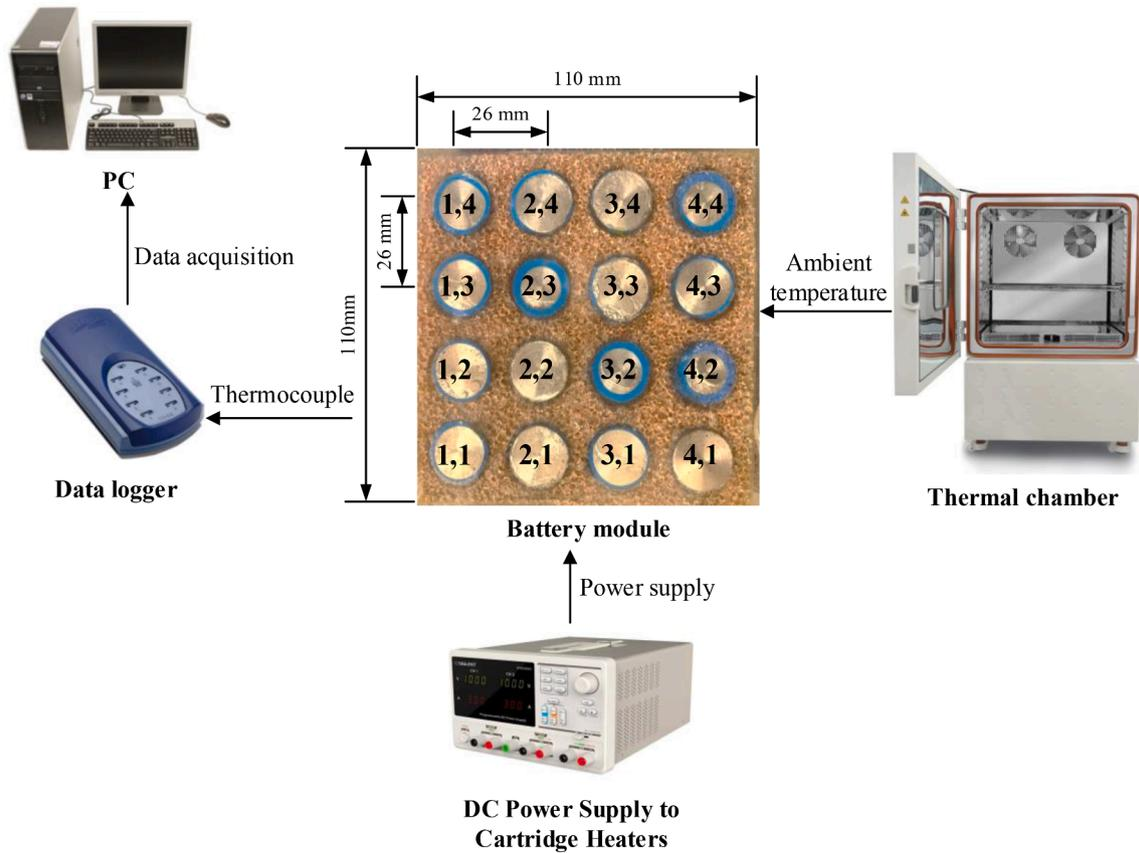
Fig. 4. Schematic diagram of the experimental setup.
