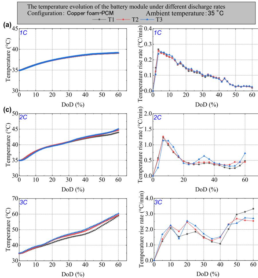
**Fig. A7.** Temperature curves of the battery module under copper foam-PCM cooling at  $T_{amb} = 35\text{ °C}$ : (a) temperature evolution of battery at 1C; (b) temperature rise rate of battery at 1C; (c) temperature evolution of battery at 2C; (d) temperature rise rate of battery at 2C; (e) temperature evolution of battery at 3C; (f) temperature rise rate of battery at 3C.
