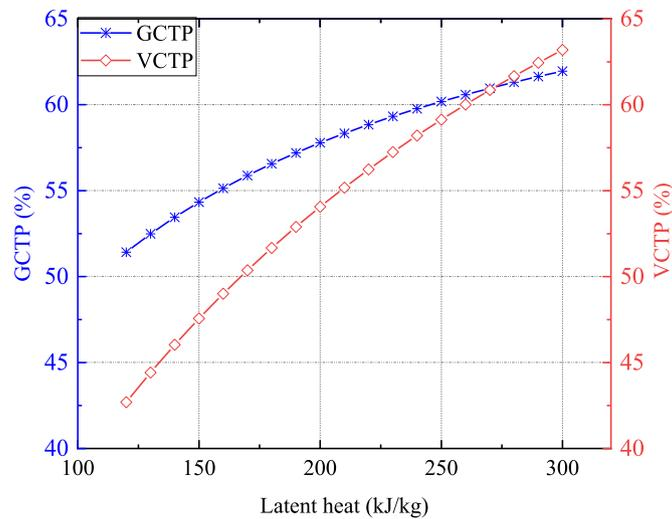
Fig. 10. GCTP and VCTP of the battery pack under various latent heat of PCM.
