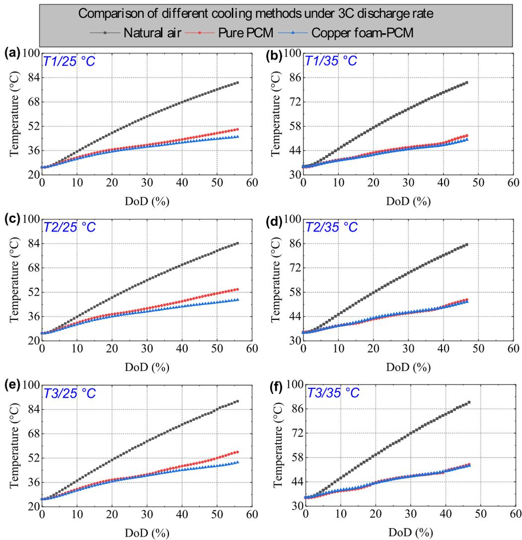
Fig. 6. The influence of different cooling methods on battery temperature under 3C discharge rate: (a) T1,  $T_{amb} = 25\text{ }^{\circ}\text{C}$ ; (b) T1,  $T_{amb} = 35\text{ }^{\circ}\text{C}$ ; (c) T2,  $T_{amb} = 25\text{ }^{\circ}\text{C}$ ; (d) T2,  $T_{amb} = 35\text{ }^{\circ}\text{C}$ ; (e) T3,  $T_{amb} = 25\text{ }^{\circ}\text{C}$ ; (f) T3,  $T_{amb} = 35\text{ }^{\circ}\text{C}$ .
