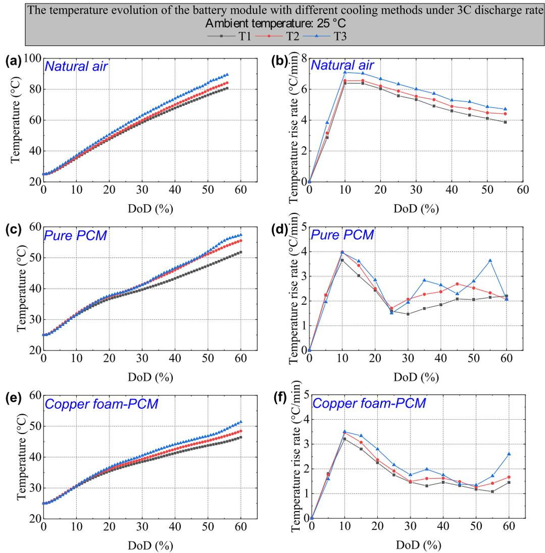
**Fig. 5.** Temperature curves and temperature rise rate of the battery module with different cooling methods under 3C discharge rate at  $T_{amb} = 25\text{ °C}$ : (a), (b) natural air cooling; (c), (d) pure PCM; (e), (f) copper foam-PCM.
