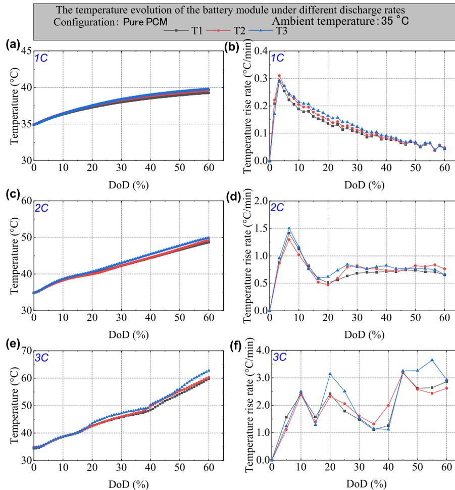
**Fig. A5.** Temperature curves of the battery module under pure PCM cooling at  $T_{amb} = 35\text{ °C}$ : (a) temperature evolution of battery at 1C; (b) temperature rise rate of battery at 1C; (c) temperature evolution of battery at 2C; (d) temperature rise rate of battery at 2C; (e) temperature evolution of battery at 3C; (f) temperature rise rate of battery at 3C.
