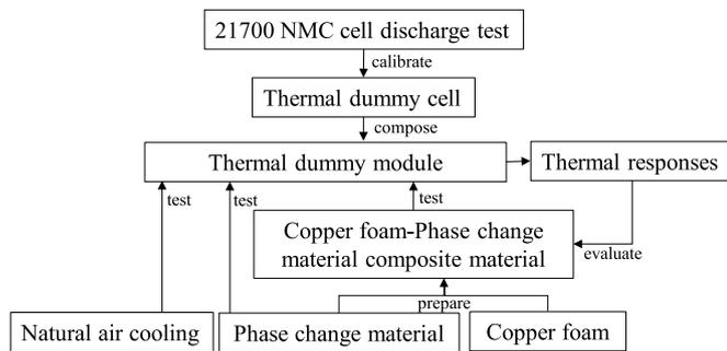
Fig. 1. Schematic diagram of the experimental study design.
