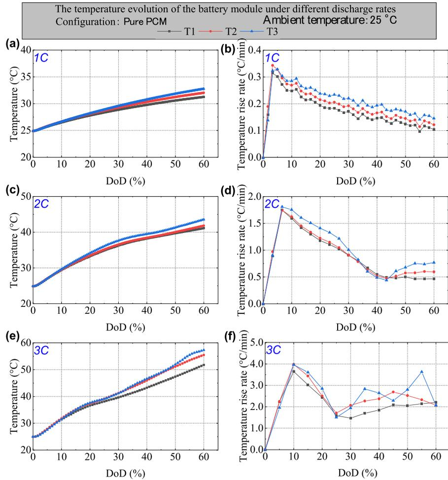
**Fig. A4.** Temperature curves of the battery module under pure PCM cooling at  $T_{amb} = 25\text{ °C}$ : (a) temperature evolution of battery at 1C; (b) temperature rise rate of battery at 1C; (c) temperature evolution of battery at 2C; (d) temperature rise rate of battery at 2C; (e) temperature evolution of battery at 3C; (f) temperature rise rate of battery at 3C.
