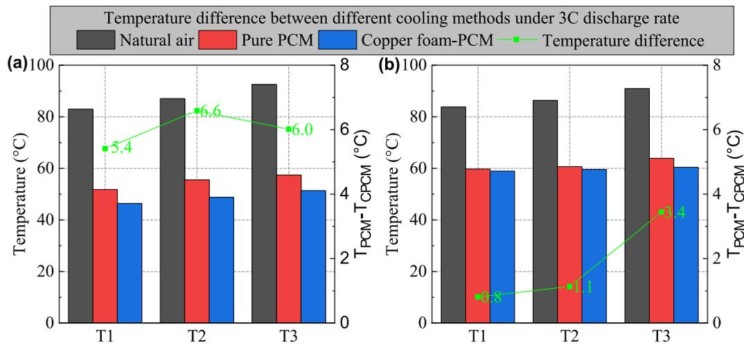
Fig. 7. Temperature difference between different cooling methods at the end of 3C discharge rate test: (a)  $T_{amb} = 25\text{ }^{\circ}\text{C}$ ; (b)  $T_{amb} = 35\text{ }^{\circ}\text{C}$ .
