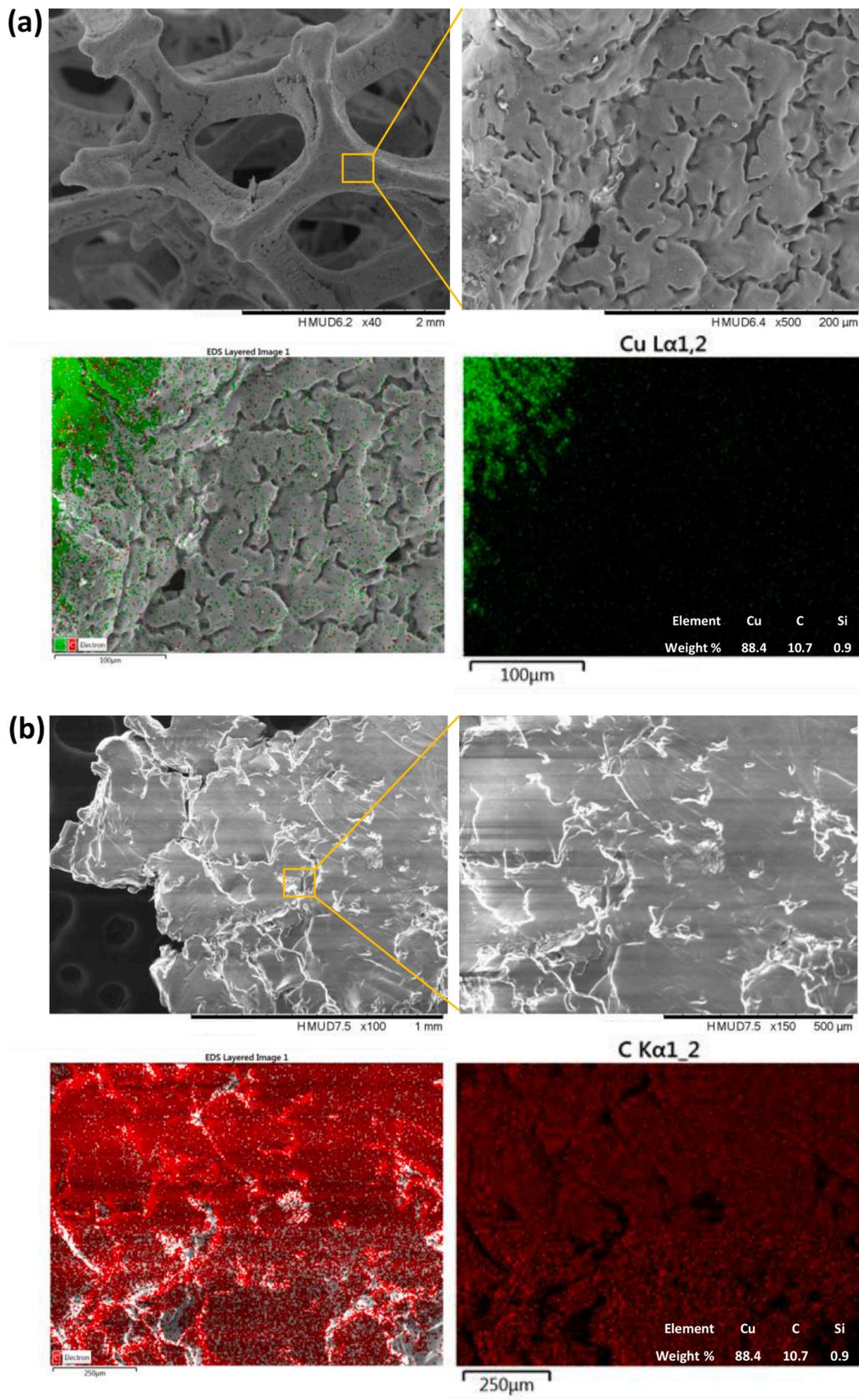
Fig. A1. SEM images of cooling materials: (a) copper foam; (b) paraffin.
