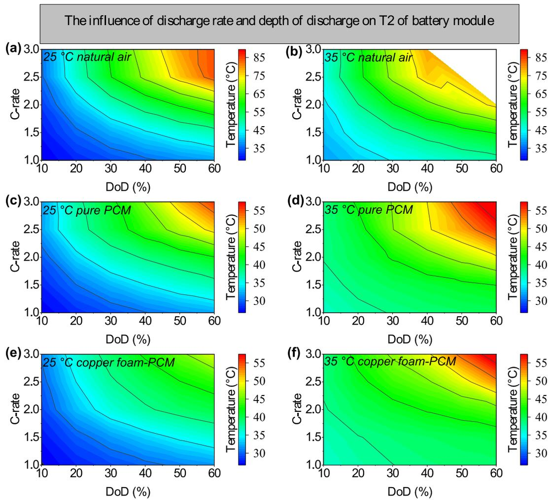
Fig. 9. Effects of discharge rate and depth of discharge on temperature evolution of battery module: (a) natural air,  $T_{amb} = 25\text{ }^{\circ}\text{C}$ ; (b) natural air,  $T_{amb} = 35\text{ }^{\circ}\text{C}$ ; (c) pure PCM,  $T_{amb} = 25\text{ }^{\circ}\text{C}$ ; (d) pure PCM,  $T_{amb} = 35\text{ }^{\circ}\text{C}$ ; (e) copper foam-PCM,  $T_{amb} = 25\text{ }^{\circ}\text{C}$ ; (f) copper foam-PCM,  $T_{amb} = 35\text{ }^{\circ}\text{C}$ .
