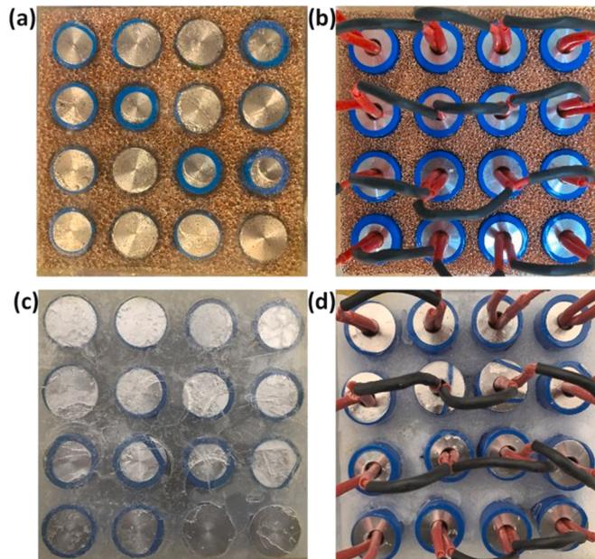
Fig. 3. Battery module with cooling material: (a) copper foam-PCM, bottom view; (b) copper foam-PCM, top view; (c) pure PCM, bottom view (d) pure PCM, top view.
