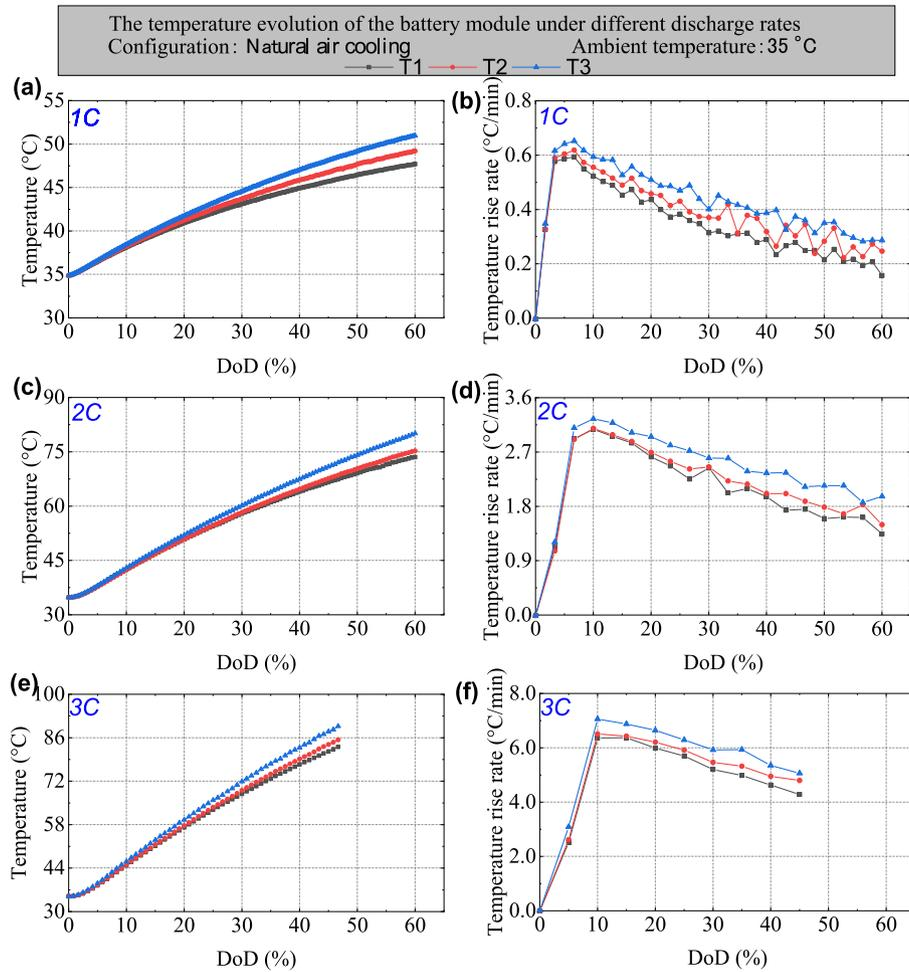
**Fig. A3.** Temperature curves of the battery module under natural air cooling at  $T_{amb} = 35\text{ °C}$ : (a) temperature evolution of battery at 1C; (b) temperature rise rate of battery at 1C; (c) temperature evolution of battery at 2C; (d) temperature rise rate of battery at 2C; (e) temperature evolution of battery at 3C; (f) temperature rise rate of battery at 3C.
