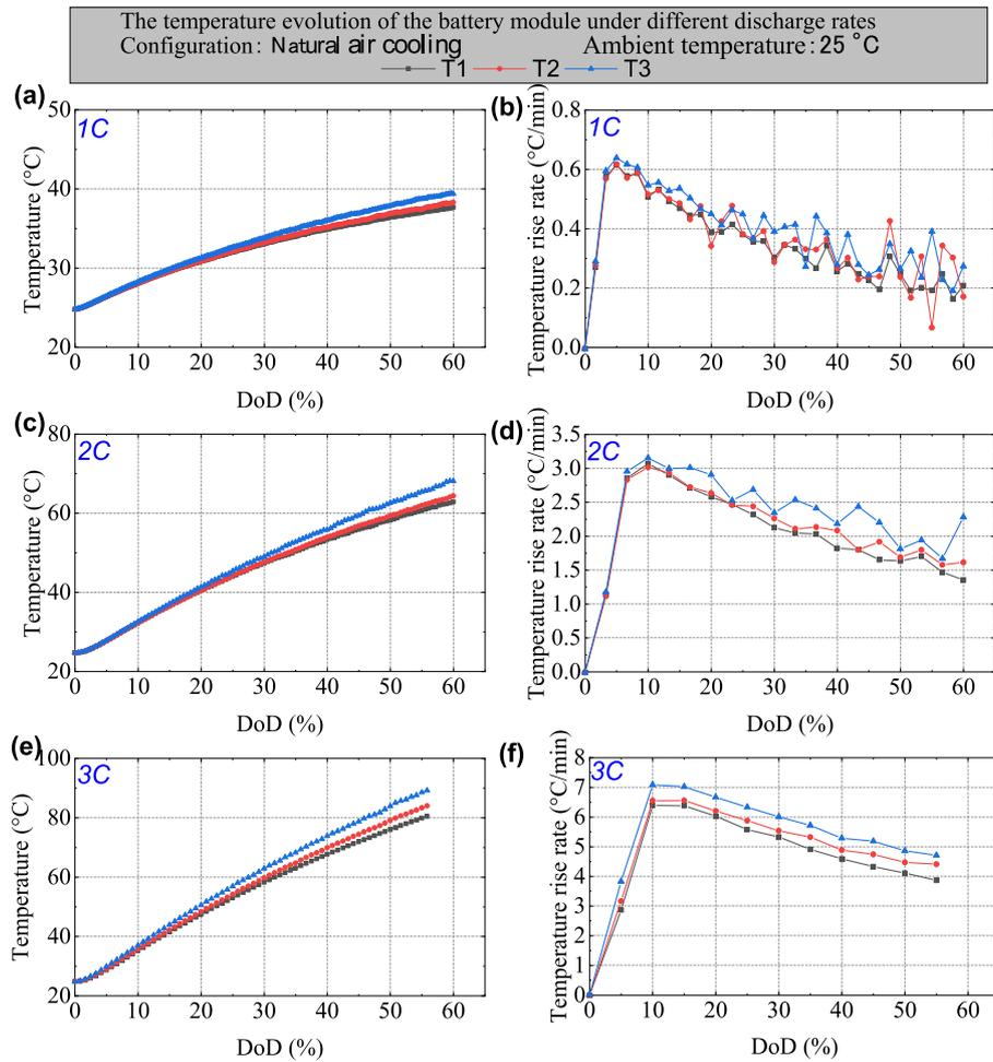
**Fig. A2.** Temperature curves of the battery module under natural air cooling at  $T_{amb} = 25\text{ }^{\circ}\text{C}$ : (a) temperature evolution of battery at 1C; (b) temperature rise rate of battery at 1C; (c) temperature evolution of battery at 2C; (d) temperature rise rate of battery at 2C; (e) temperature evolution of battery at 3C; (f) temperature rise rate of battery at 3C.
