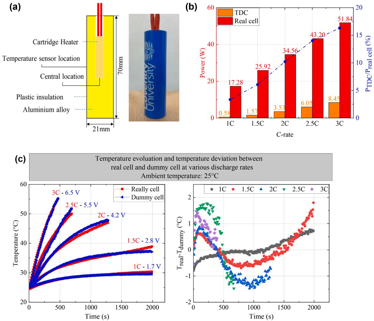
**Fig. 2.** The experimental setup for TDC: (a) Longitudinal section and practicality diagram of TDC; (b) Electrical power consumption of the TDC and real cell; (c) Temperature evolution of TDC and real cell at various discharge rates.
