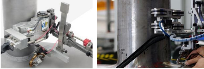
FIGURE 1 EXAMPLE STATE OF THE ART NOZZLE WELD INSPECTION SYSTEMS, LEFT: JIREH NAVIC - 3-AXIS NOZZLE SCANNER [8], RIGHT: PHOENIX NOZZLE SCAN [9]
