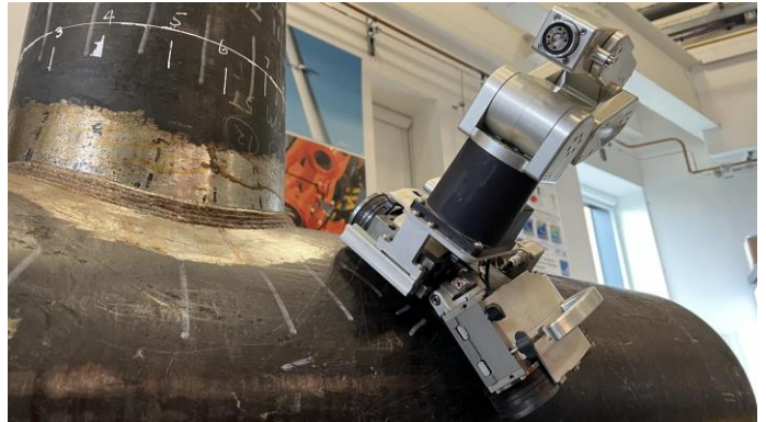
FIGURE 4 CURRENT MAGNETIC CRAWLER, UTILISING AN ARTICULATED BASE
