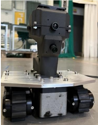
FIGURE 5 CRAWLER WITH AN ARRAY OF SIX CAMERAS
