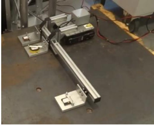
FIGURE 8 PROTOTYPE GUIDED WAVE OCCUPANCY GRID MAPPING CRAWLER
