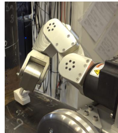
FIGURE 13 PLATFORM PERFORMING MOCK INSPECTION OF THE SADDLE WELD
