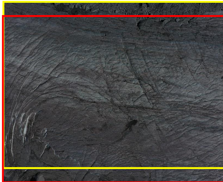
Figure 2.34: Typical lateral overlap between two images (red and yellow outline). (Image from Flight 2, 27/8/16).
