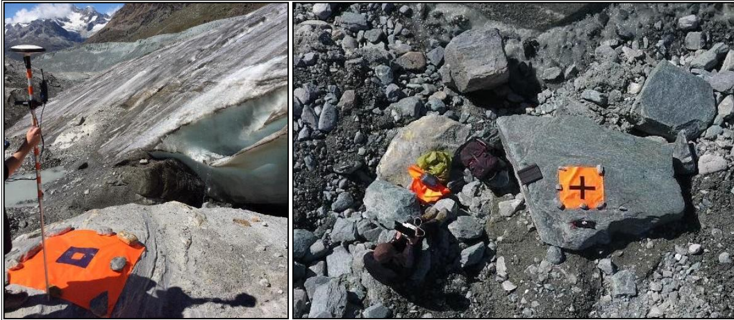
Figure 2.35: Different GCPs shapes and sizes used between 2016 (left) and 2017 (right).
