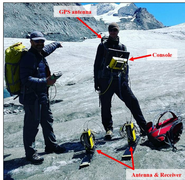
Figure 2.22: Pulse Ekko GPR set up at Findelengletscher.
