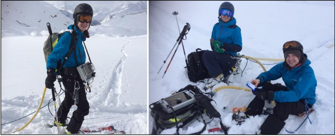
Figure 2.20: MALA GPR device with 25 MHz Antenna coil - Findelengletscher February 2017.
