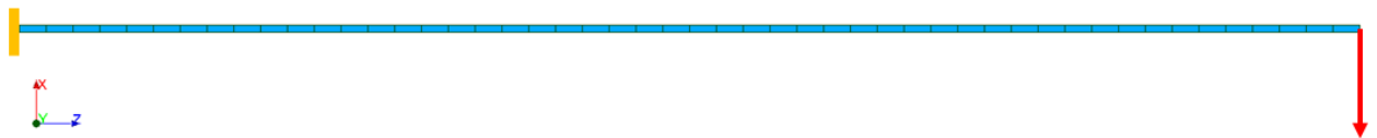
Figure 6.2: Diagram of the cantilever beam testcase. A single nodal force on first harmonic (cos) is applied at the free end of the beam, in the middle.
