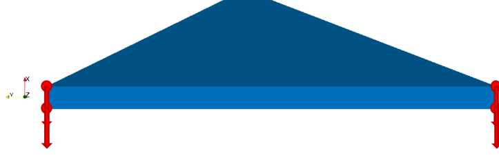
Figure A.2: Diagram of the cantilever beam test case for the appendix, highlighting the distribution of the excitation force. The total excitation magnitude is 2N .
