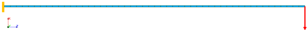
Figure A.1: Diagram of the cantilever beam testcase for the appendix, same as in Figure 6.2.
