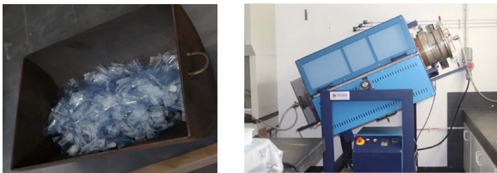
Figure 1. Small pieces of waste PET and the rotative furnace used for char and activated carbon production.
