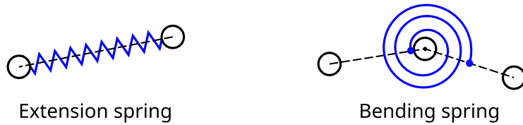
Figure 4. Types of springs used in mass-spring models for flexible insect wings.
