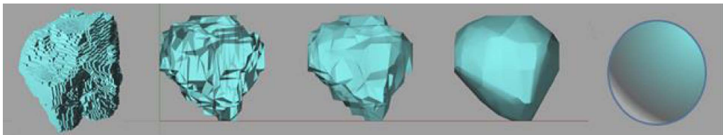
Figure 2. Digital transition of the particles used in the digital packings, from digital reconstruction of Berea sandstone grain to a spherical particle.
