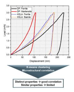
Fig.1 Representative load and depth curves of the tested DP and HSLA steel and its individual constituent.
