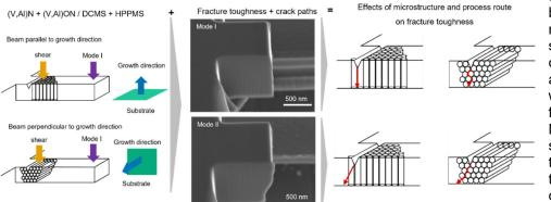
In the course of this work by comparing mode I and mode II beam bending, we show that HPPMS coatings exhibit denser and stronger interfaces which leads to a higher fracture toughness. Nevertheless, DCMS showed higher fracture toughness values due to the observations that the crack stopped at underdense regions in the microstructure and needed to be newly initiated.
