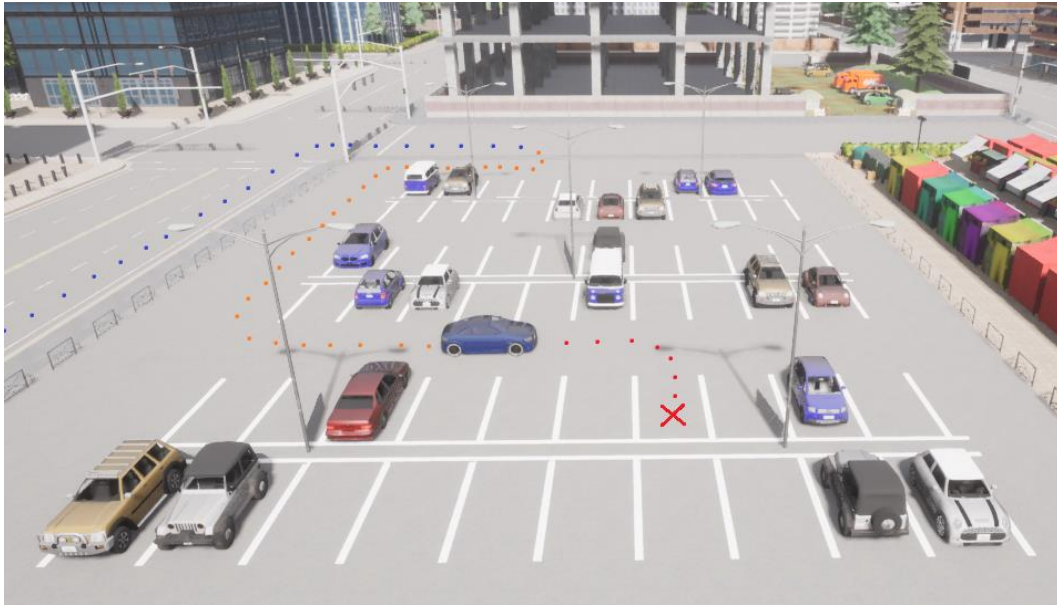
Figure 23. Example of the three motion planning phases for parking inside the car park.
