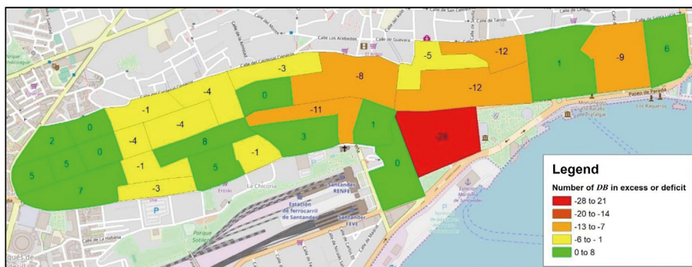
Fig. 6. Number of delivery bays excessive or lacking compared to the current number when applying the methodology during peak hours.
