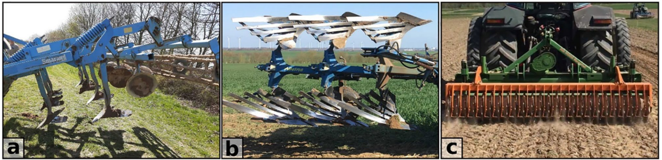
Figure 2. Implements used within tillage experiments: (a) chisel plough, (b) mouldboard plough, and (c) roller.
