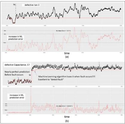
Figure 5. Illustration of the technique employed to detect (a) significant change in bushing tan  $\delta$  and (b) significant change in bushing capacitance C1. The sudden error increase in the prediction of the model is used to detect the fault.
