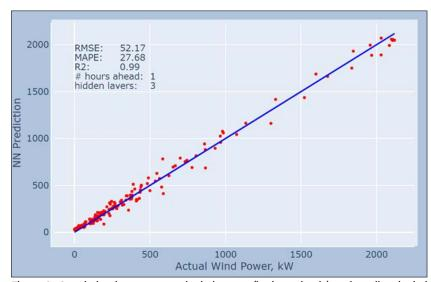
Figure 3. Correlation between actual wind power (horizontal axis) and predicted wind power by the machine learning algorithm. Predictions were made for 1h ahead, short-term forecast.
