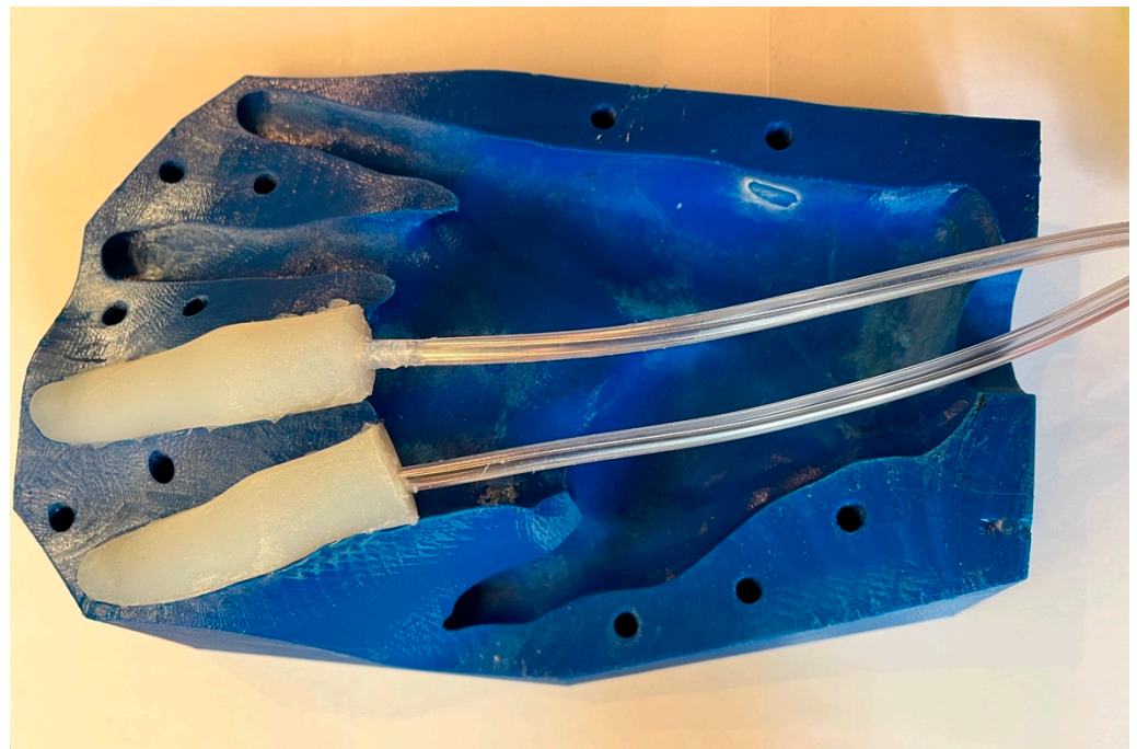
Figure 7. Palmar part of the mold of Hazubski et al. [20] with inserted placeholder fingers and tubes for creating cable routing through the hand.
