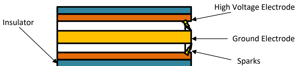
Figure 5.3: Schematics of a cylindrical spark plug
