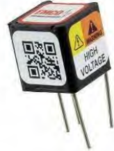
Figure 4.4: EMCO Q20-5 0.5W 2kV. Sourced from: Digikey
