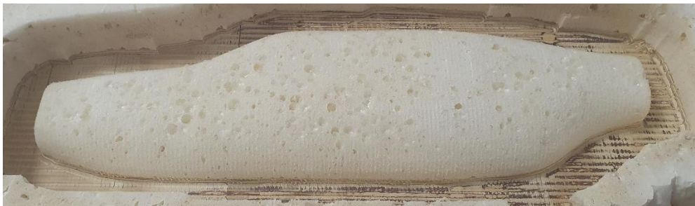
Figure 5.22: VTOL fuselage produced utilising combined additive and subtractive manufacturing
