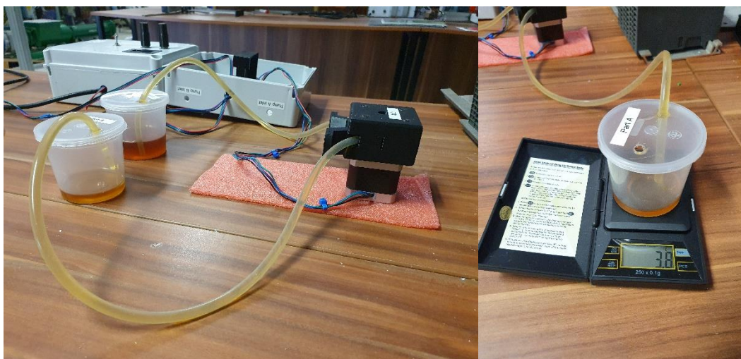
Figure 5.7: Experimental procedure to determine the mass flow rate of both products
