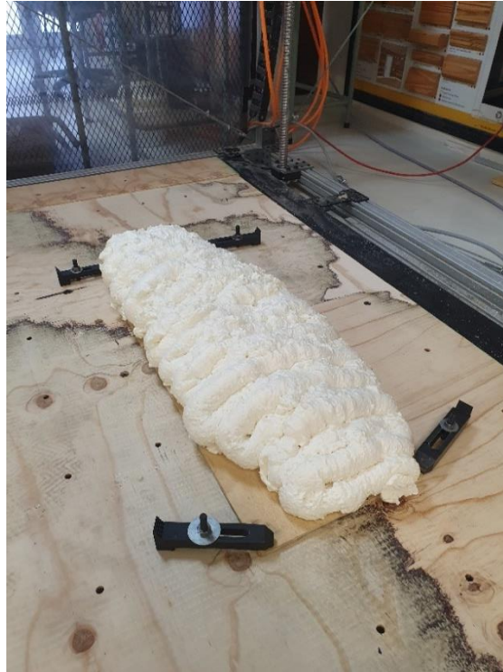
Figure 5.20: Additively deposited fuselage model
