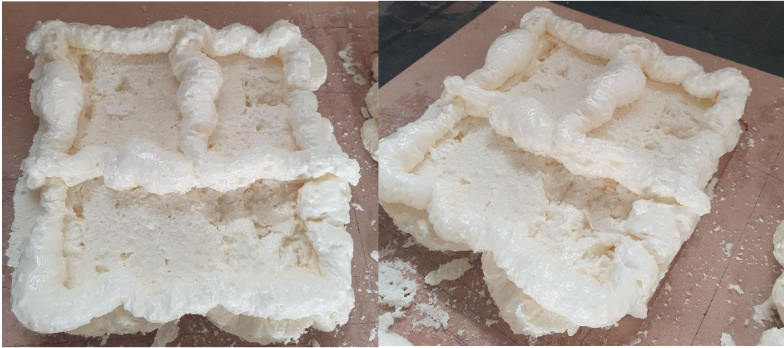
Figure 5.45: PU house model additively deposited along the walls
