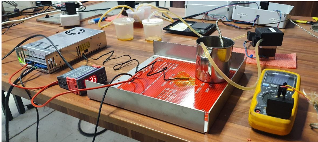
Figure 5.10: Temperature control system utilised to decrease the viscosity of part A
