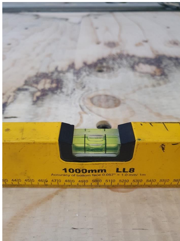
Figure 3.9: Face milled sacrificial bed
