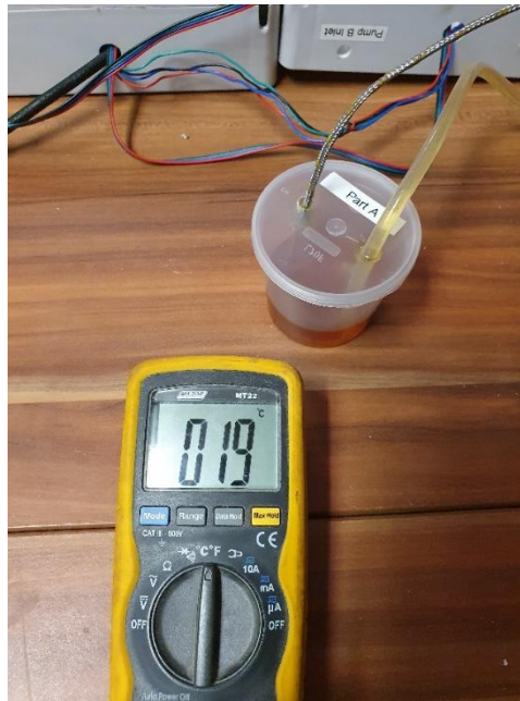
Figure 5.8: Thermocouple used to measure the temperature of the product
