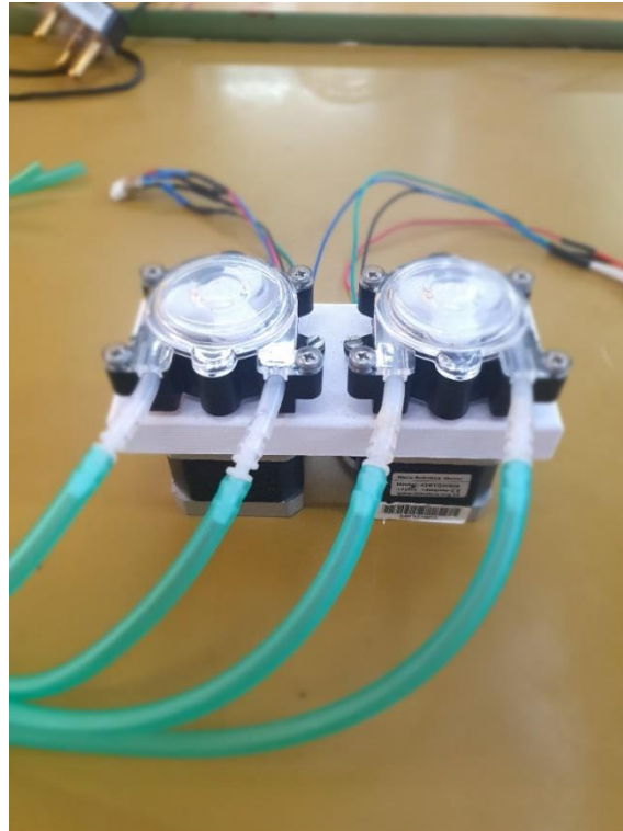
Figure 3.14: Assembled splined stepper motor dosing system
