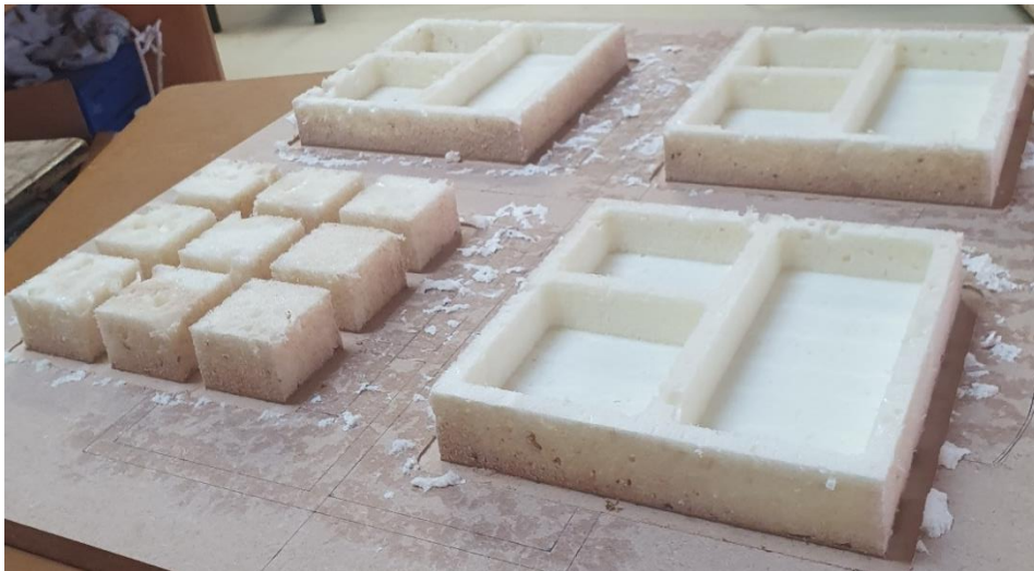
Figure 5.41: Three house models and nine calibration cubes produced using the developed HM system
