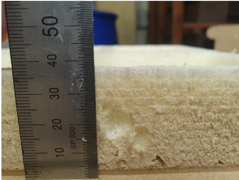
Figure 5.32: Example of a coarse surface finish
