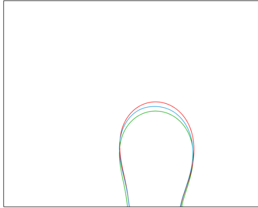
Figure 5-14. Droplet shape comparison between YS, piecewise linear and MPI for jetting mode with frequency 61.7 MHz at approximately 10 ms. Green line depicts YS, Red line illustrates piecewise linear and Blue line shows MPI.
