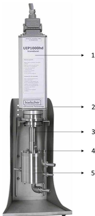
Figure 13 The UIP1000HdT system consisting of a transducer (1), ST2 support (2), booster (3), sonotrode (4) and flow cell (5). Image obtained from [[https://www.hielscher.com/es/i1000\\_p.htm](https://www.hielscher.com/es/i1000_p.htm)].
