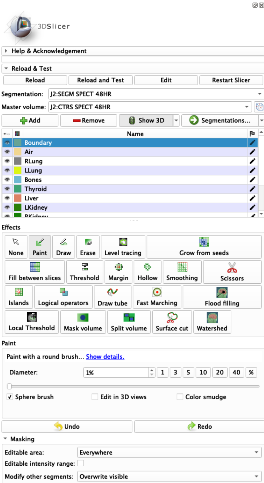
Figure 3.6: Segment Editor module of 3D-Slicer
