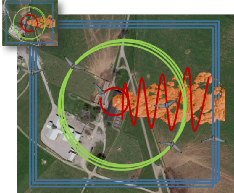
Figure 1.1: A visualization of how a mobile sensing platform can be used in a contaminant leak scenario is shown. As the platform passes through the contaminant it is able to measure the local atmospheric properties to help aid in estimating the contaminant trajectory.
